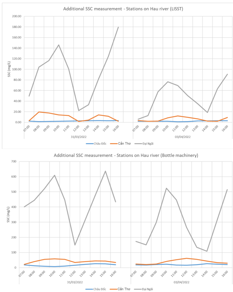
Figure 2-22: SSC data in dry season at stations on Hau River with two different measurement techniques.
