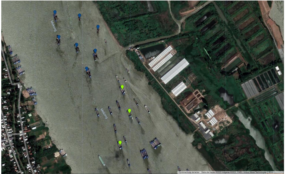
Figure 3-36, Manually classified active barges with cranes vs. double moored transport vessels (which show the same geometrical characteristics in S2 imagery), zone-example.
